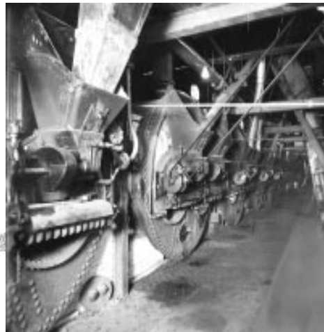
Underground installation of boilers, shafting and belting was designed for Salts Mill with the aims of providing a safer working environment and an integrated approach to the production of textiles. Source : RCHME
